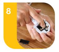
Never replace a fuse with one for a higher voltage.
