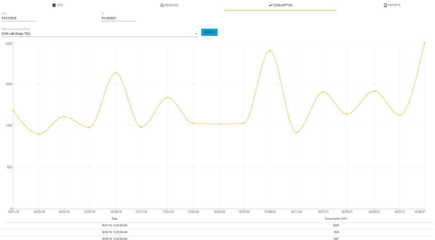
By selecting a different measuring channel the consumption/generation of all available measuring channels and components can be displayed.
