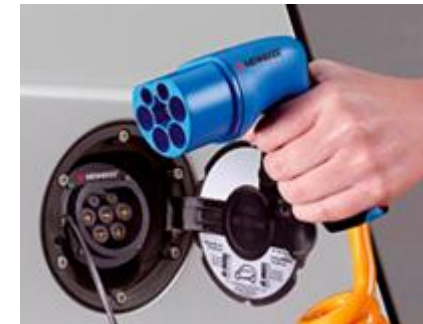
TYPE 2 (AC Charging) 43kW max
